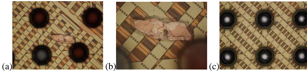
Fig. 2. (a) and (b) show optical images of a wafer surface with Cu metal residue, (c) optical image of wafer cleaned using a formulation with OneStep technology and without metal residue after field metal etch.
